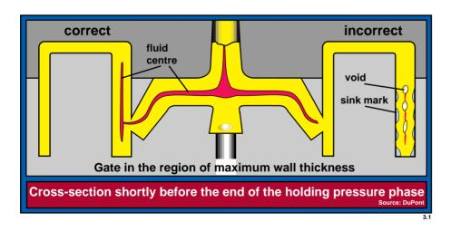
The position of the gate is decisive for the flow front profile and the effectiveness of the holding pressure and, as a result, for the strength and other properties of the moulded part.
