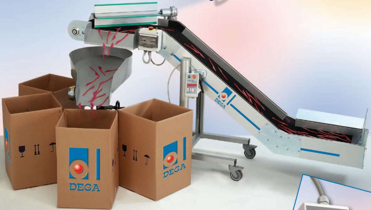
The **SERVER** is an ancillary device that is used in conjunction with a conveyor belt or a robot to allow collection and distribution of a pre-determined number of mouldings from a moulding machine into a box or bag with a minimum of a floor space.
